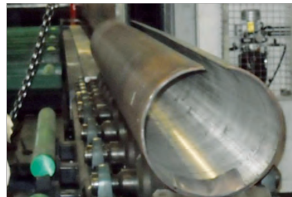
7. Lamiera clad formata a C (open pipe). 7. C-formed clad plate.
