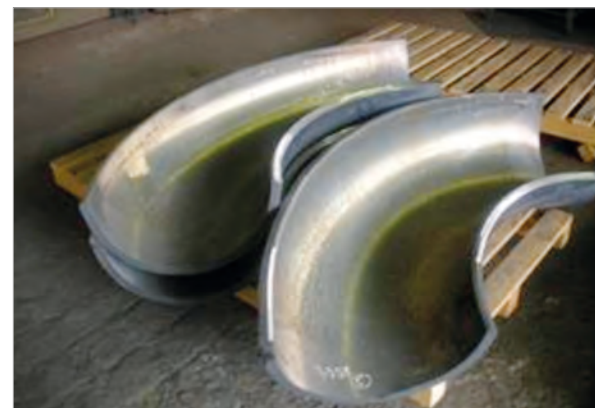
11. Gusci prodotti da lamiera clad mediante formatura a caldo. 11. Shells manufactured from clad plate through hot forming.
