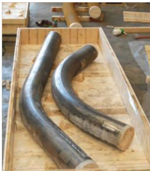
14. Curve piegate mediante processo a induzione. 14. Bends obtained through an induction process.
